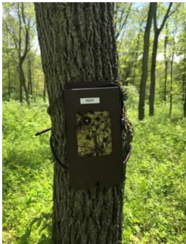
Figure 1. 4: Picture of Anabat Swift mounted to a tree in the field.
