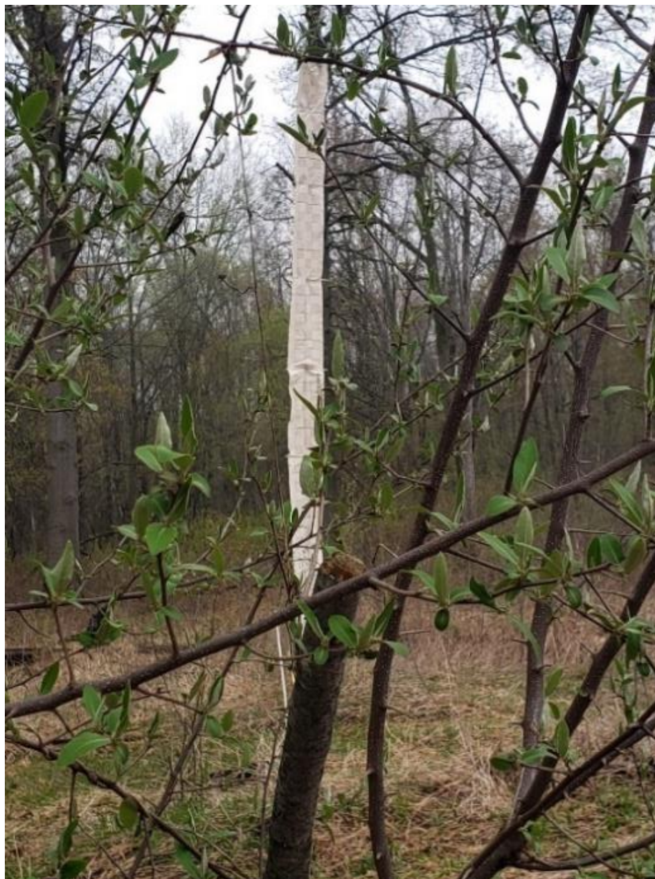
Figure 2.1. Clutter board used for measuring vegetation clutter at multiple height levels
