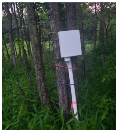
Figure 1.2. Acoustic monitoring set up for (a.) stationary monitor stations with monitor inside lockbox) and (b.) transects
