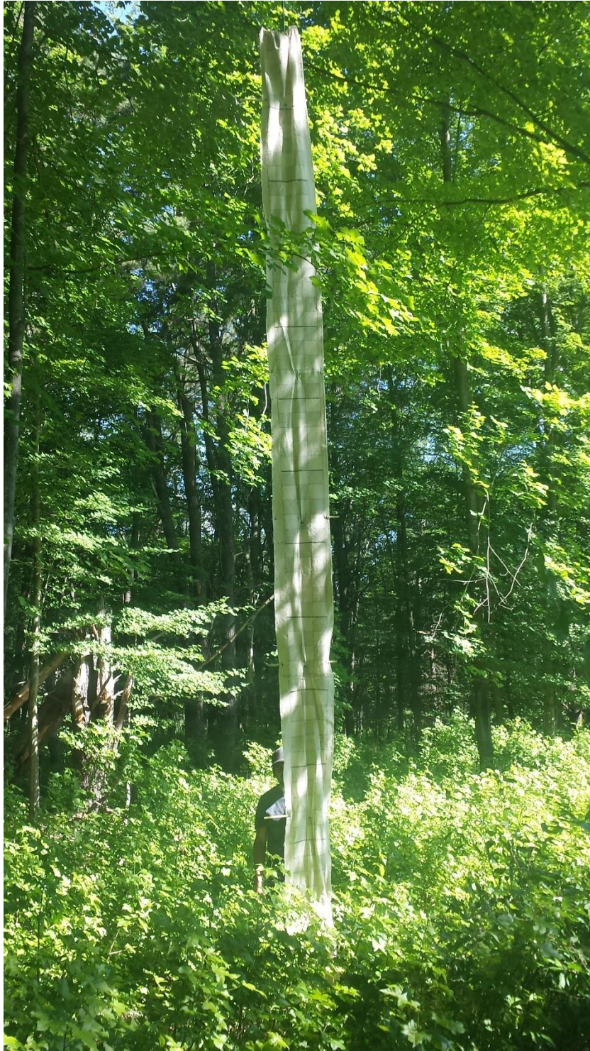
Figure 5: Example of use of a scatterboard to measure vegetation densities at varying heights.
