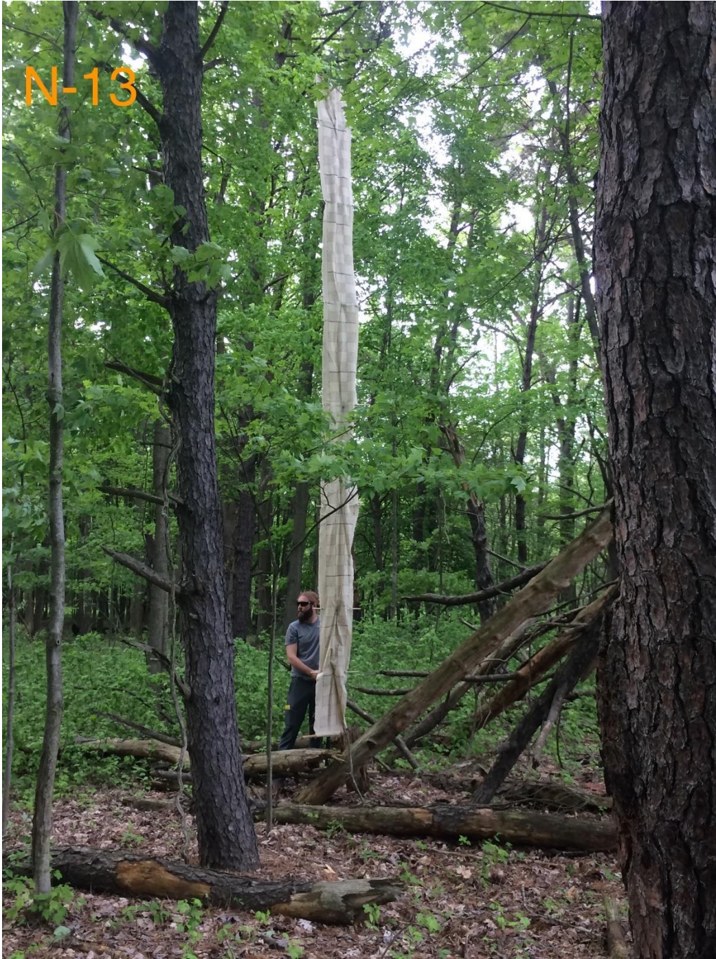
Figure 15: Example of scatterboard being used for vegetation density measurements. The board was set up 15 m away from the stationary site and measured in all four cardinal directions then averaged for the site.
