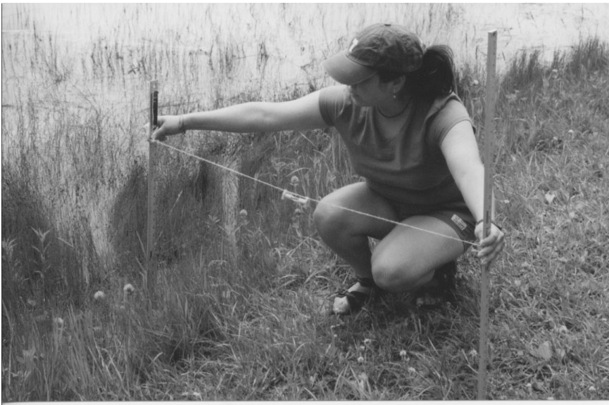
Figure 12. Measuring the slope of the pond bank within 1 meter of its edge.
