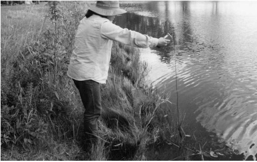
Figure 11. Temperature and pH measurements taken in the field at each site using a portable meter.
