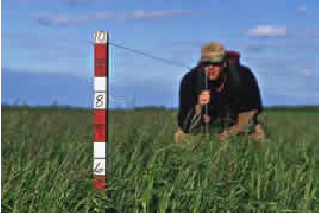
Figure 6: How a Robel pole is used. This Robel pole measurement would be 5.5 dm. The top half of the red 5 dm band is visible, and the bottom 5.5 dm of the pole is completely obscured from view.
